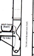
The main characteristic of this WC is that it is easy to keep clean, has no parts needing maintenance, can be demounted easily, and can be transportable without the risks attached to porcelain.
