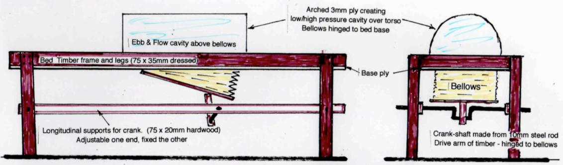
Crank rotates approx every 8 seconds in oiled hardwood 'bearings'
